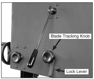
**Figure 18.** Release lock lever before adjusting tracking.
